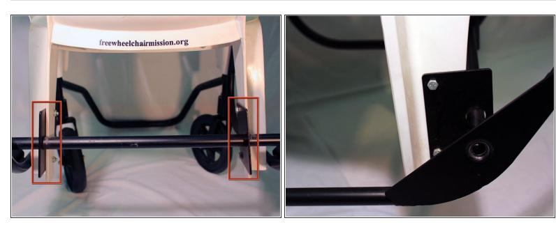
Locate the two baseplates on the back of the wheelchair holding the axle in place
