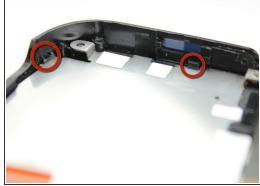
• Locate the four tabs above the keyboard. The following steps will demonstrate how to remove the metal plate from the tabs, which will reveal the keyboard.
