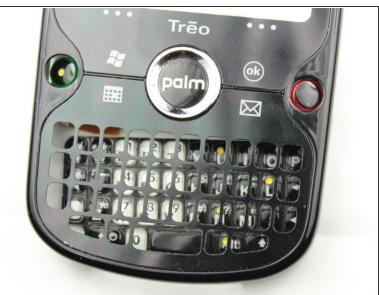
Rotate the phone cover so that the face of the cover is facing up as shown in picture two. The keyboard should fall out from the keyboard holes.
