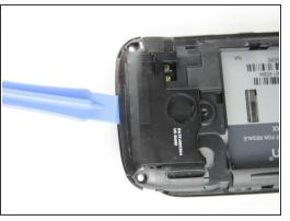
Use a plastic opening tool to remove the small panel on the top of the phone by prying underneath the black plastic around the camera.
