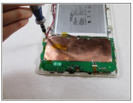
Unscrew the four 3mm Phillips #00 screws found in each corner of the motherboard.
