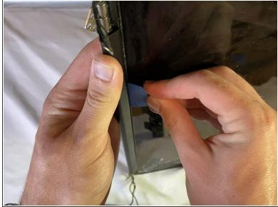
Loosen the adhesive between the hinge cover and screen by inserting an opening pick and sliding it across
