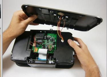
Use a plastic opening tool to pry off the white ZIF connector joining the wires to the motherboard.
