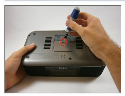
Remove the 10 mm-length, 5 mm-head screw using a Phillips #1 screwdriver.
