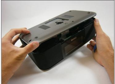
1 The bottom cover is attached to the back cover by two plastic clips. Don't use excessive force.
