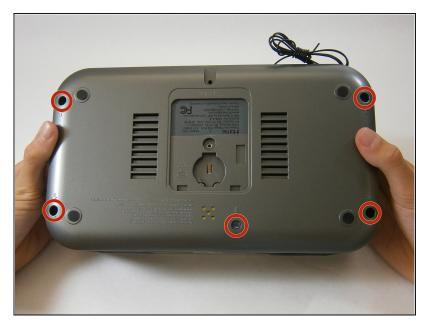
Unscrew five 17 mm-length, 6 mm-head screws using a Phillips #1 screwdriver.
