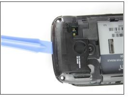
Use a plastic opening tool to remove the small panel on the top of the phone by prying underneath the black plastic around the camera.
