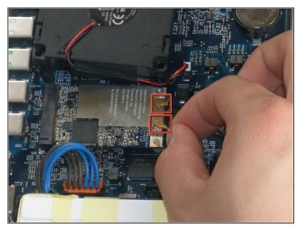
Pry the AirPort antenna cables straight up from their sockets on the logic board.
