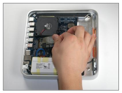
Cautiously lift the AirPort card and pull it straight away. Slide it from its socket on the logic board.
