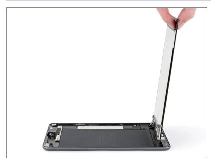
• To avoid stressing any cables, hold the screen perpendicular to the frame.
