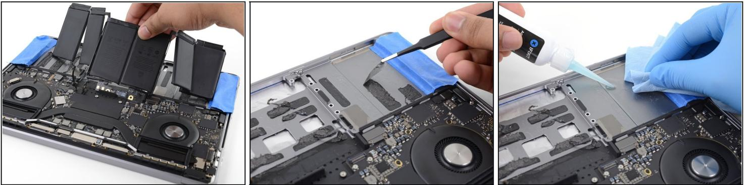
**⚠** Before you remove the battery, ensure that the [battery connector is sufficiently raised](#) and not in the way of the battery board.
