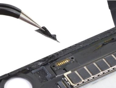
• Use a pair of tweezers to remove the sticker covering the magnetic sensor solder pads.
