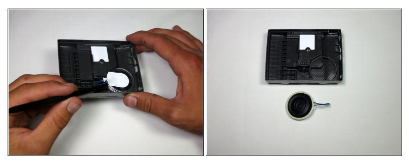
• Detach speaker from casing and insert new, functional speaker.
