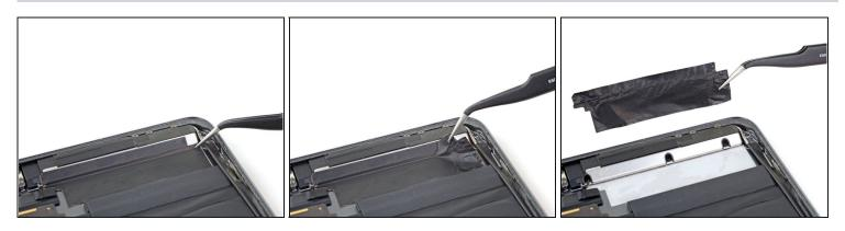
• Use a pair of tweezers to remove the tape covering the left speaker screws.
