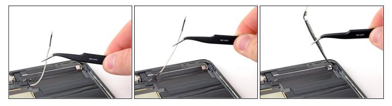
• Use a pair of tweezers to peel the left antenna cable away from the rear case.
