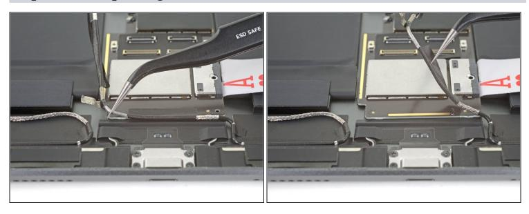
• Use a pair of tweezers to peel the right antenna cable away from the logic board.
