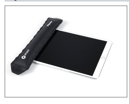
Apply heat to the top edge of the iPad for about two minutes, or until it's slightly too hot to touch comfortably.
