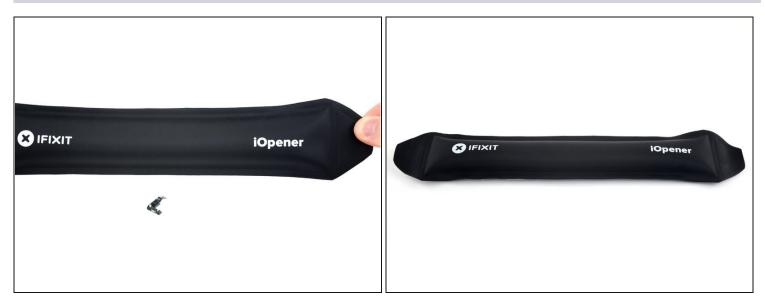
• Apply a heated iOpener to the power button assembly for thirty seconds.
