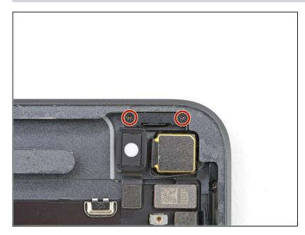
Use a Phillips screwdriver to remove the two 4.3 mm-long screws securing the power button bracket to the rear case.
