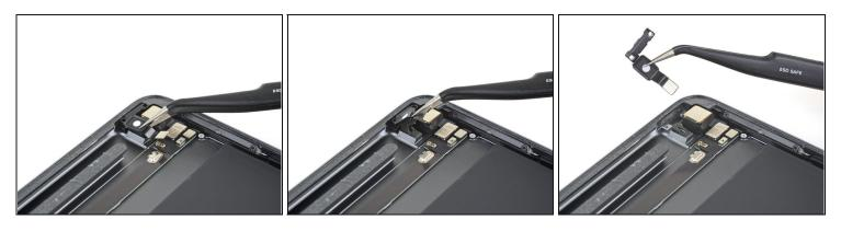
Use a pair of tweezers to peel the power button assembly away from the rear case.
