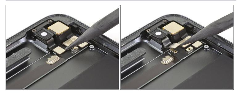
• Use the pointed end of a spudger to disconnect the front camera cable by lifting straight up on the press connector.
