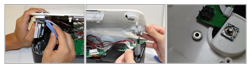
• Use a plastic opening tool to pry the black connections away from the top casing.
