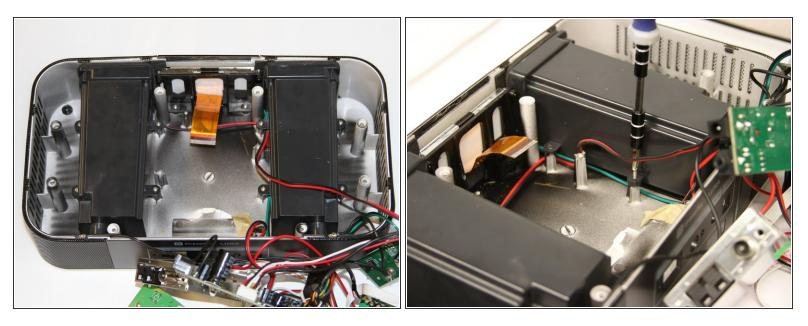
• Unscrew four 7mm Phillips screws from the base of each speaker unit.
