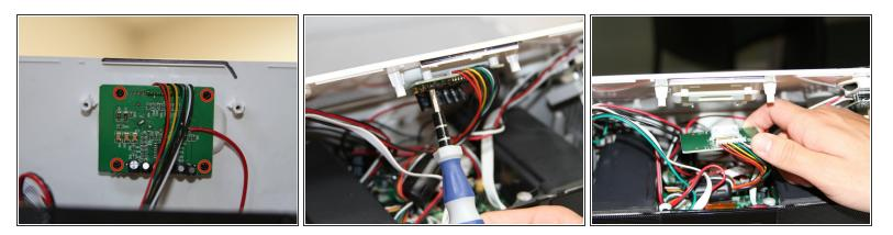
Unscrew the four black 7mm screws with the Phillips #1 screw driver that hold the middle circuit board to the top case.
