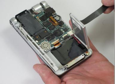
Pull up on the black tab on the battery pack to reveal the power cord.
