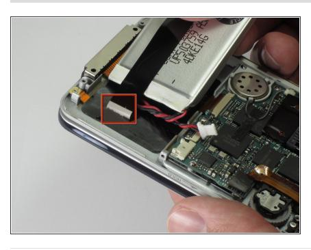
Gently peel back the adhesive to completely disconnect the battery pack from device.
