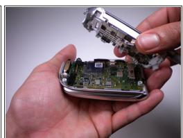
While removing the back panel, take out the rubber cover on each side.
