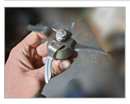
Wash the assembly with detergent and water to remove any dust, grease or grime. The repair is now complete!
