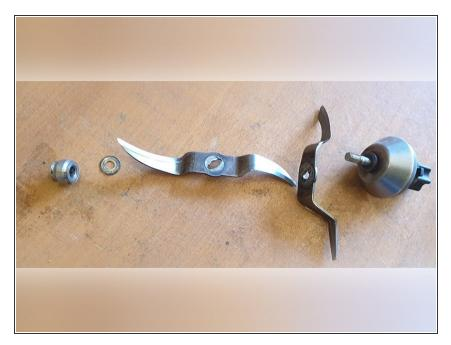
Once the head is loosened and removed take apart the blade assembly. Note the blade orientation.
