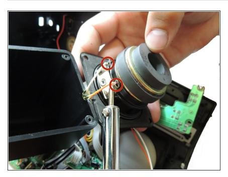
Unsolder the two wires that connect to the speaker.
