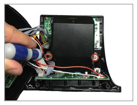
Remove the two 12.0mm screws holding the speaker to the iHome with a Phillips #1 screwdriver.
