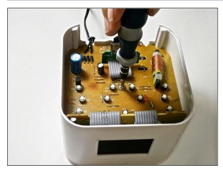
• Using a Phillips #1 screwdriver, remove the screw found in the middle of the board.
