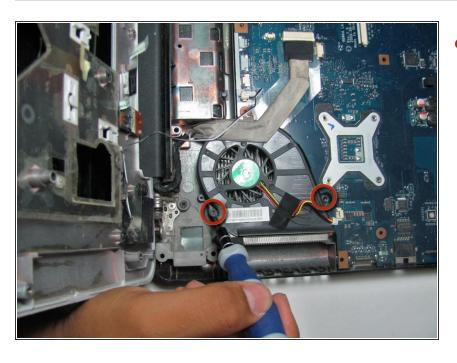
Remove the two 6mm screws with a Phillips #00 screwdriver.
