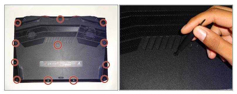
Remove eleven screws from the back of the laptop using a Phillips #0 screwdriver.
