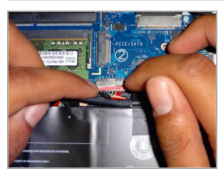
Reconnect the battery pin by reinserting the connector back into its slot.
