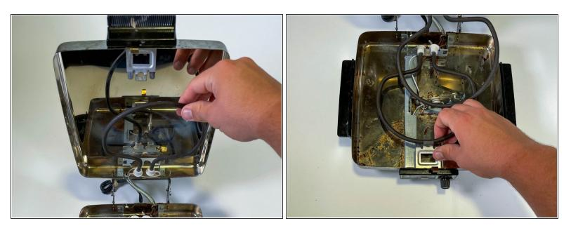
• Remove the heating elements from their respective housings (the bottom one is not able to be removed completely as it is fused to a piece of metal).
