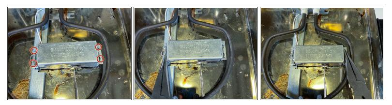
Use pliers to twist the metal tabs holding down the thermostat housing.
