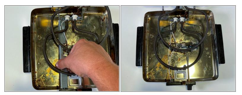
• Remove the housing from the wiring along the bottom of the grill.
