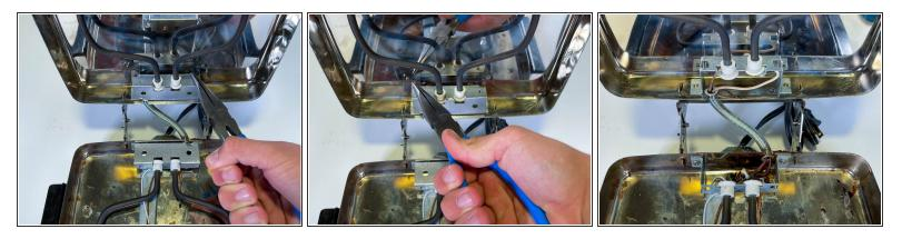
• Use a pair of Large Needle Nosed Pliers to twist the metal tabs holding the plate housing the top heating element connections and remove the plates.
