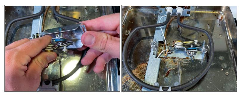
• Remove the thermostat housing.
