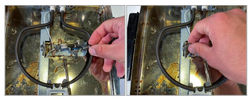
• Remove the thermostat housing springs.
