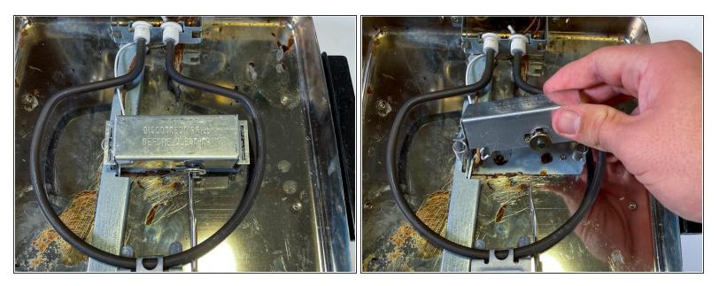
• Lift up the thermostat housing and detach it from the temperature control arm, then remove the washers at the end of the temperature control arm.
