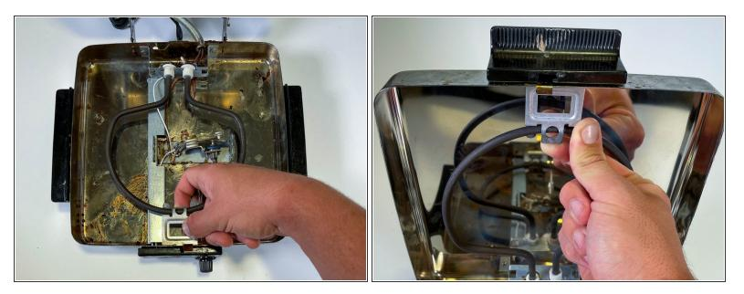
• Bend up the brackets holding down the heating elements.
