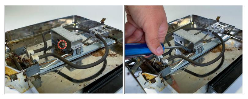
Use a 4 mm Flathead screwdriver to remove the 11.4 mm screw in the back of the thermostat housing.
