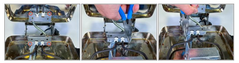
Use a pair of Large Needle Nosed Pliers to twist the metal tabs holding the plate housing the bottom heating element connections and remove the plate.
