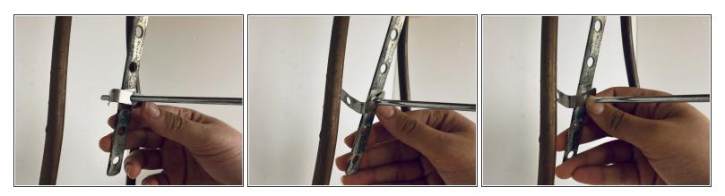
• Disconnect the lift rod for the drain plug by pushing it off the metal rod.
