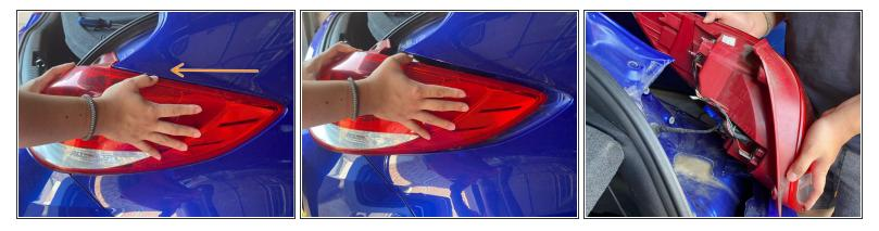
Using both hands, carefully pull the brake & tail light off.
