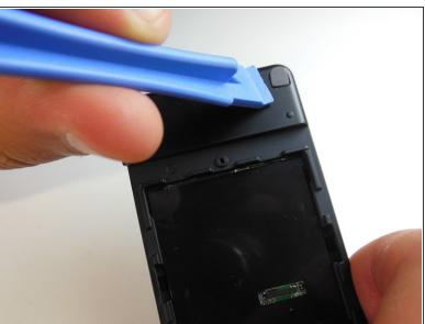
Remove the four corner plastic covers on the back of the device using the plastic opening tool.
