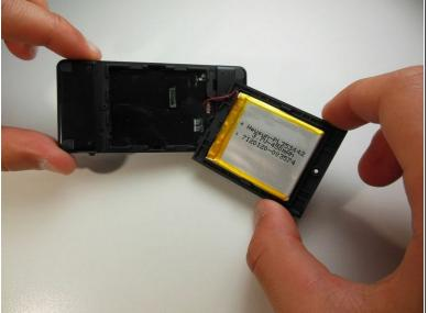
Detach the back cover by carefully pulling up and out on the back plastic casing.
