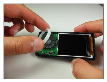
Remove the white plastic ring from around the scroll wheel with your fingers.
