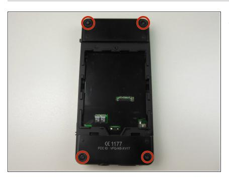
Using a Philips #00 screwdriver remove all four 4.5mm corner screws located underneath the corner pads.
