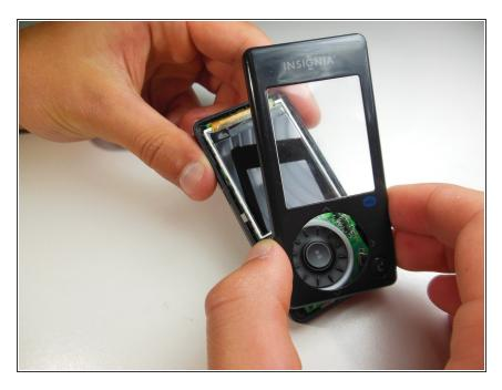
Once the front cover is loose, use your fingers to remove the front case cover for a new installation.
