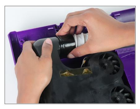
Place and twist the hose cuff onto the fan opening.
