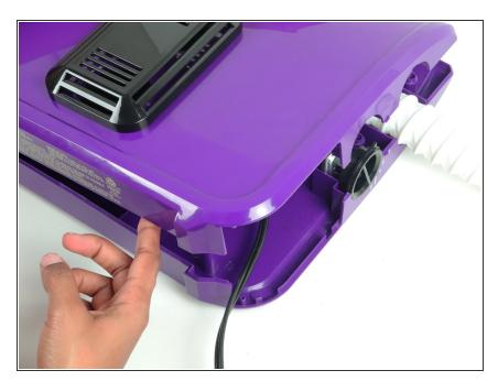
Place the hair dryer's front cover on top of the back cover, leaving a finger's width space for the next step.
