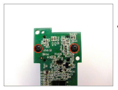
Remove the two 8mm Phillips#0 screws on the back of the motherboard.
