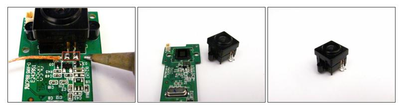
• Remove the camera from the motherboard by desoldering the two connections as shown.
