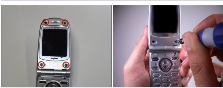
Use the Tri-Wing Y1 screwdriver to unscrew the now uncovered four 0.5 mm screws.
