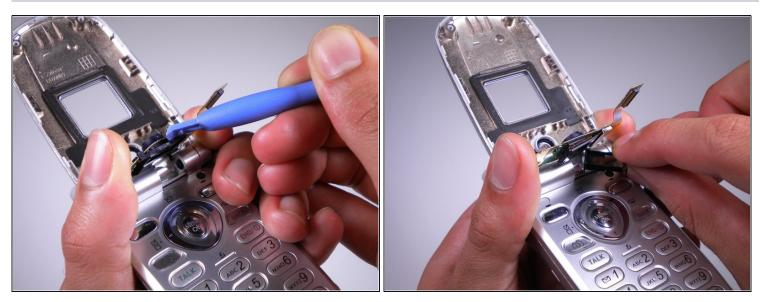
• Use the opening tool to take off the black plastic frame around the camera lens.
