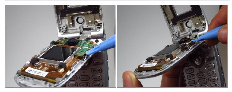
• Use plastic opening tool to lift the chip on the right side.
