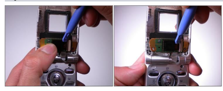
• Use the plastic opening tool to flip the ZIF connector to the right.
