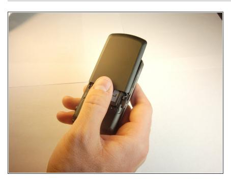
Push the battery cover from the indentation and slide the battery cover away from phone to remove battery cover
