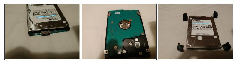
As the drive has a USB port soldered directly to its logic board, instead of a converter board in between, disassembling this device seems to be pointless unless the hard drive is being used for parts.
