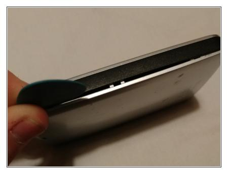
Slide your spudger along the gap in the casing you made in the previous step, continuing to open the device.
