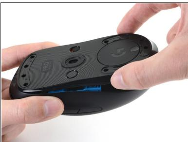
⚠ Don't try to remove the lower case from the upper case yet. They are still attached by the battery cables and input cable.
