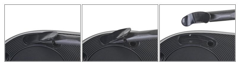
Slide the spudger under the length of the left lower mouse foot to cut through the adhesive and detach it from the mouse.
