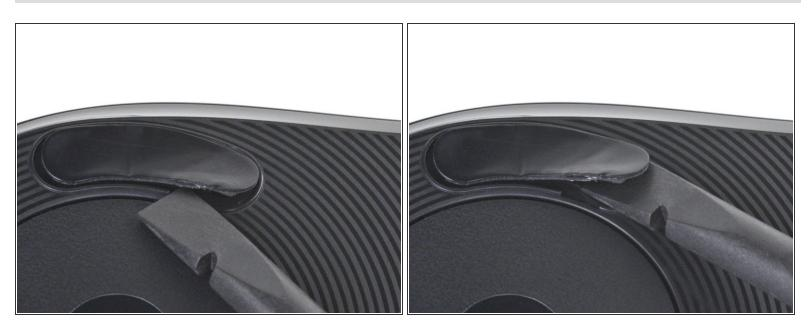
Insert the flat end of a spudger under the left lower mouse foot.
