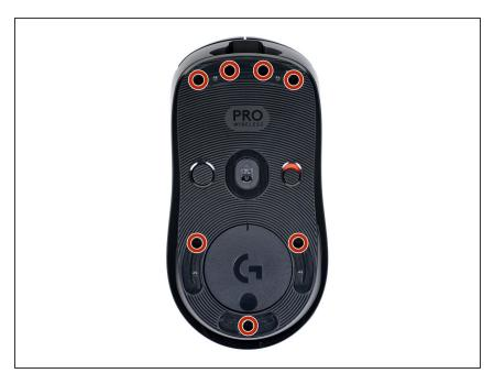
Use a Phillips screwdriver to remove the seven 4.4 mm-long screws securing the lower case.
