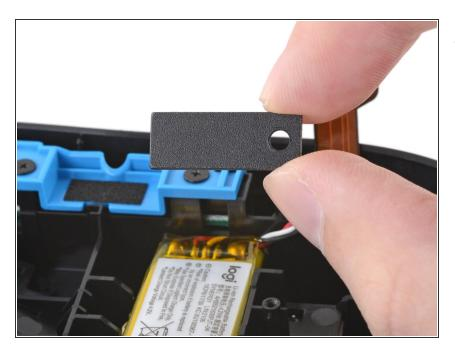
Remove the battery plate from the battery.
