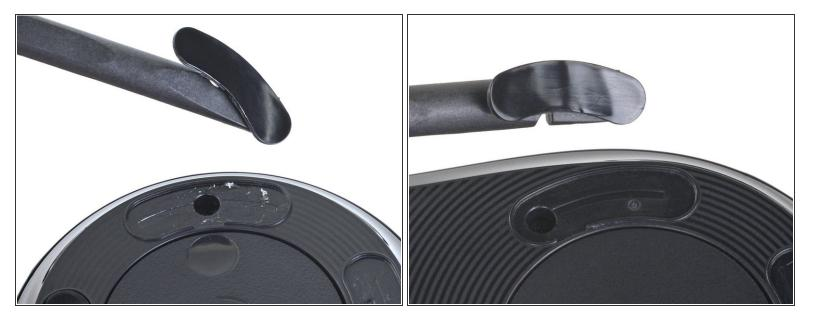
Repeat the procedure to remove the two remaining lower mouse feet.
