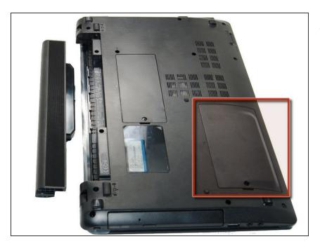
Locate the HDD compartment bottom of the laptop
