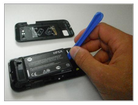
Insert the opening tool between the battery and the battery holder and wedge the battery out.
