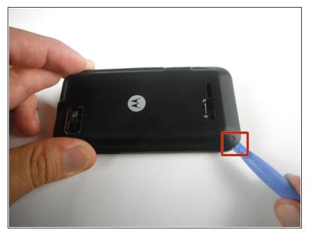
Wedge the plastic opening tool in between the back cover and the body of the phone in the opening denoted by the arrow.
