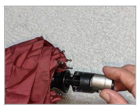
Verify that the button is firmly fixated to the metal ejector.
