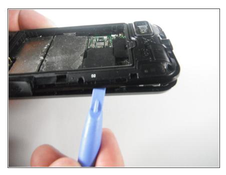
Wedge the plastic opening tool between the plastic layer and the shiny front cover.
