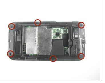
Use the Torx T4 screwdriver to remove the six 3 mm screws from the back case.
