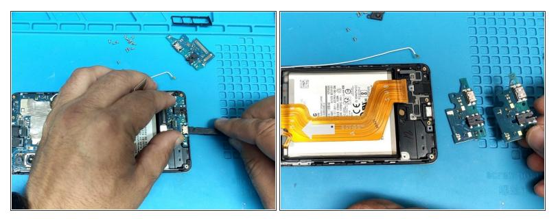
• Carefully pry out the old charging board, and put in the new one.
