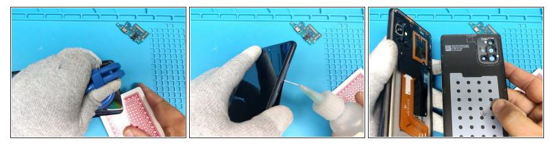
• Now we are going to separate the back cover. First, warm up the device to soften the adhesive, then use a plastic spudger to open up the rest of the device.
