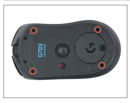
Use a Phillips screwdriver to remove the four 5.4 mm screws securing the two halves of the mouse together.
