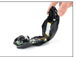
⚠ Don't completely separate the two halves yet—they're still tethered together by a delicate cable.
