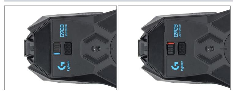
Before you begin, flip the mouse's power switch into the red OFF position.
