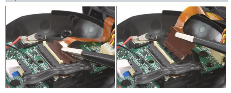
Use a pair of blunt nose tweezers or your fingers to slide the interconnect cable out of its socket.
