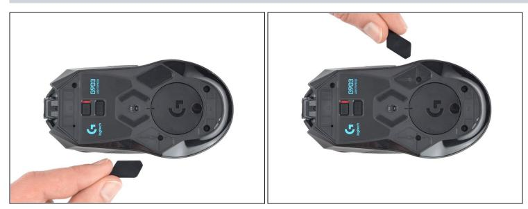
Repeat the previous mouse feet removal procedure and remove the two pentagonal mouse feet on the left and right side.
