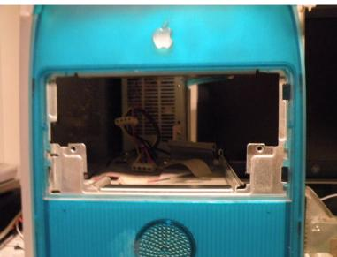
Removing the drive cage:
