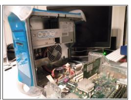
Start By Disconnecting the computer, and lifting the tab on the side of the computer, and lowering the side panel.
