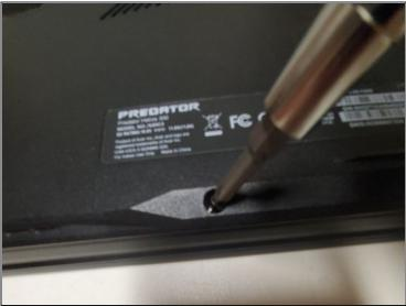
• Remove the eleven black 7.0 mm screws using a Phillips #00 screwdriver.
