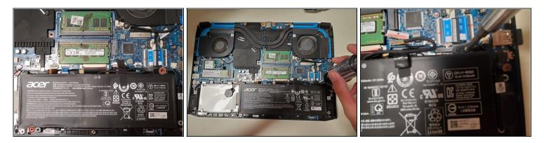
• Remove the two 4.0 mm golden screws using the Phillips #00 screwdriver.
