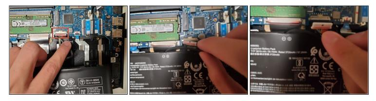
Disconnect the battery connector.
