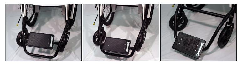
• To change the footrest's position, repeat the previous steps but move the footrest bar to the preferred position by lining up the footrest bar with the holes on the sides of the frame
