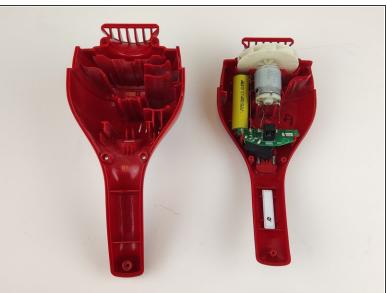
Pry open the two halves of the case.
