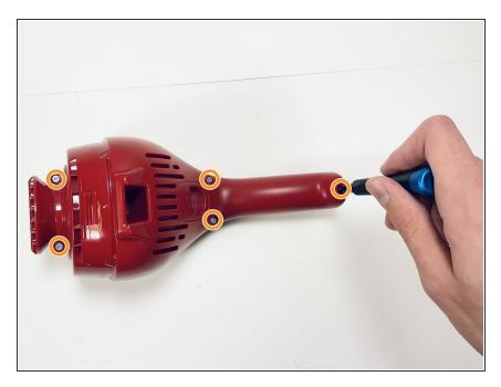
Remove five screws from the handle using a Phillips #1 screwdriver.
