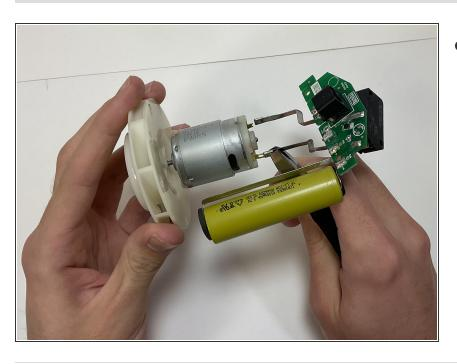
Using a pair of pliers, insert the metal prongs of the new motor into the PCB.
