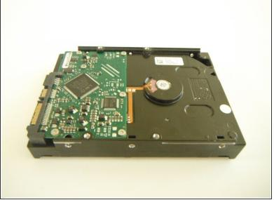
Unscrew the four 5mm screws on both sides of the hard drive using the Phillips #1 screwdriver and then remove the hard drive from the case.
