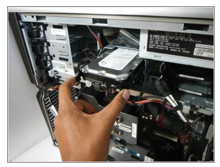
Push the tabs on both sides of the hard drive bracket towards each other and slide the hard drive up and out of the hard drive bay.
