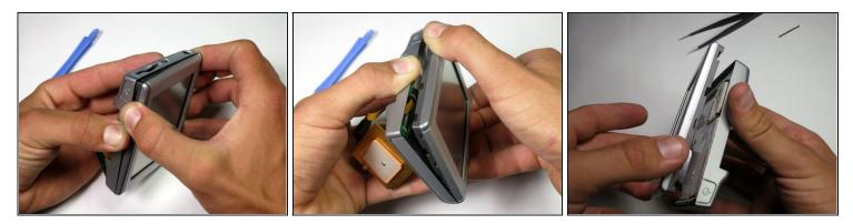
• Detach the front display from the back panel of the device.
