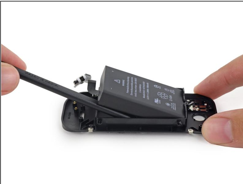
**⚠ Exercise extra caution here. Lithium ion batteries can be dangerous if punctured or bent.**
