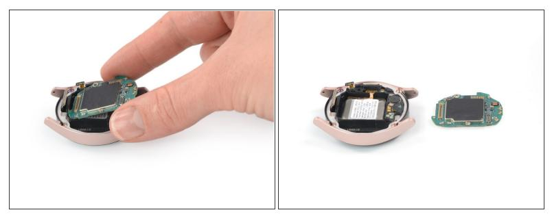
Use your fingers to lift the motherboard out from the watch assembly towards the bottom of the watch.
