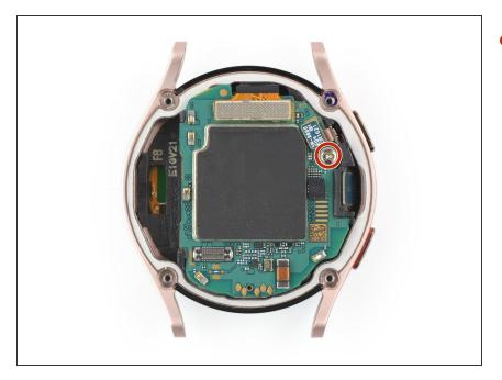
Use a Phillips screwdriver to remove the 4.4 mm-long screw securing the motherboard.
