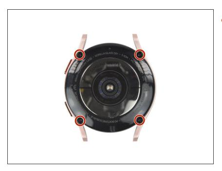
Use a Tri-point Y000 screwdriver to remove the four 4.0 mm-long screws.
