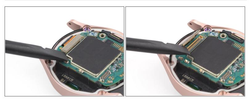
• Use the flat end of a spudger to disconnect the display flex cable.
