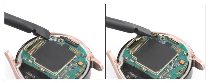
• Use a spudger to disconnect the flex cable of the crown buttons.
