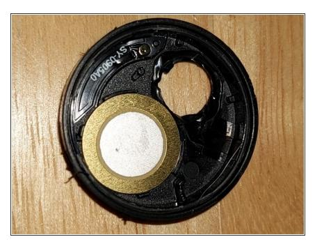
Hidden away in the top casing is a piezoelectric speaker.
